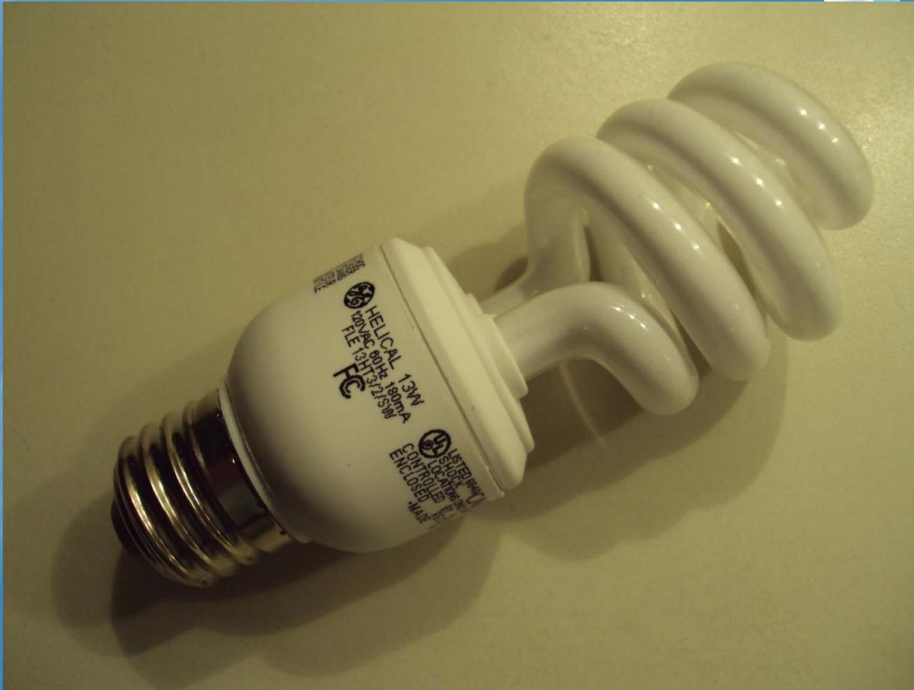
This lamp, which has micro amounts of Mercury, has EPA handling procedures.
